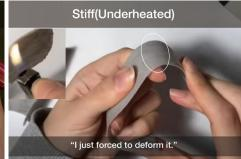
**Issue 8.** When users insufficiently heat the target parts, they force them to deform. In the worst case, the target parts may break down.
