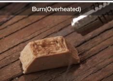
**Issue 6.** When users overly heat the target objects, the object's surface could be burnt.
