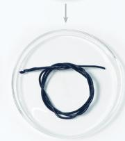
**3D Filaments** We put the coated pellets into the DIY level filament extruder\*\*. We set the extruder's temperature to 55 °C. Finally, we extruded filaments from the extruder, which have a uniform 1.75mm thickness.
