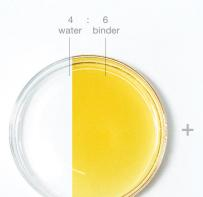
Binders We made a mixture of water and a commercialized watercolor binder\*. A higher volume ratio of the binder makes the ink too viscous and increases the thickness of the applied layer. In contrast, if the binder ratio is too low, the coating thickness becomes too thin and it hardly adheres to the target surface.
